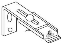
Standard wall mount installation brackets are adjustable and provide 1/2" to 1 1/2" wall clearance. Determine the height for the top of the bracket (measured from the floor) by adding 1/2" to the blind height including the headrail. When installed, louvers will clear the floor by 1/2".
