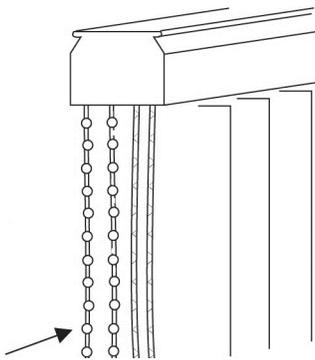
Pull the metal bead chain once in each direction, rotating the louvers from front to back. This step will align all of the louvers.
