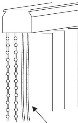
Alternatively pull the nylon cords to ensure that the blind traverses smoothly in both directions.
