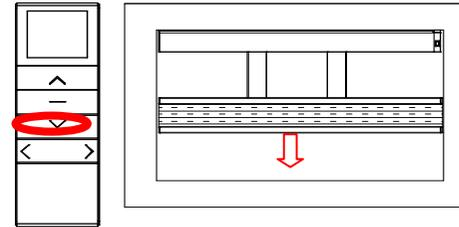
\* When reach the bottom, the bottom rail will stop and the middle will go up.
