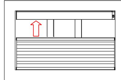
\* When middle rail meet the head rail, it is drop limit.
