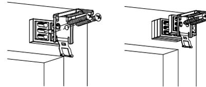
\* For shallow mounting, using flat head screw to secure the bracket in 45°.
