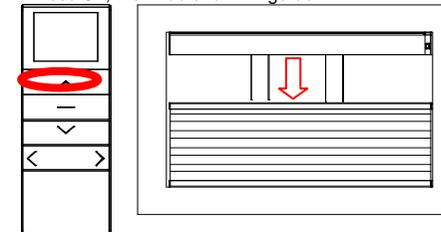
\* When the middle rail reach the bottom, the bottom rail & middle rail will go up together.
