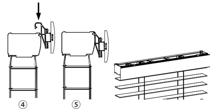
Remove the valance together with valance clip plugs away from the receptors before installing the blind. **Leave the receptors on the headrail.**
