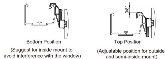
If the valance return is needed, join the valance return with valance by valance return connector first, and then attach the valance together with valance returns to the headrail.
