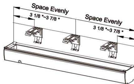
Allocate min. distance from wall face to the backside of the brackets. Peel off the double-sided adhesive tape on the bracket and stick the bracket at the marked location. Use two 1 1/4" mounting screws to secure bracket. Use wall anchors for drywall or plaster wall.
