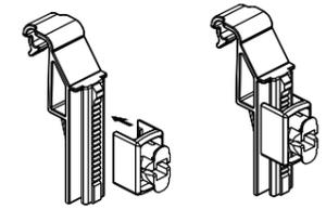
Attach the valance clip plug and receptor into the channel on the backside of the valance. Attach the valance return if needed. Hook the valance clip receptors onto the headrail and space them evenly.
