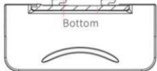
2. Position the handle hook B on the rib of bottom rail front side, like drawing ①
