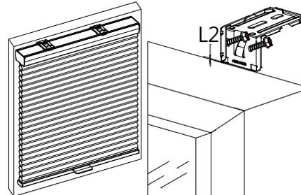
\* For shallow mounting, use 1pc or 2pcs of flat head screw to secure the bracket as below.
